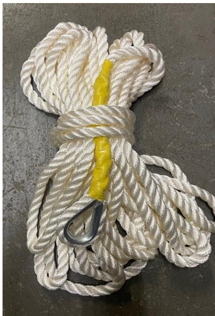
Figure 3: Lifting rope with eye splice and thimble eye
